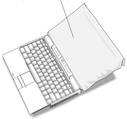
Place a soft, dry, clean cloth over the display to protect it from scratches.
